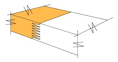
WWPA's quality control procedures for structural-glued end-jointed (i.e. finger-jointed) lumber ensure that it will meet the performance capabilities of solid-sawn lumber recognized under all model building codes. End-jointed lumber can be used interchangeably with solid-sawn lumber of the same size, grade and species.
