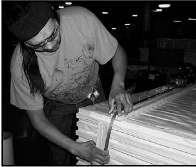
Ian Tohet (Madras Plant 7) bands an outbound unit with polyester strapping, which is cheaper and easier to handle than steel.
